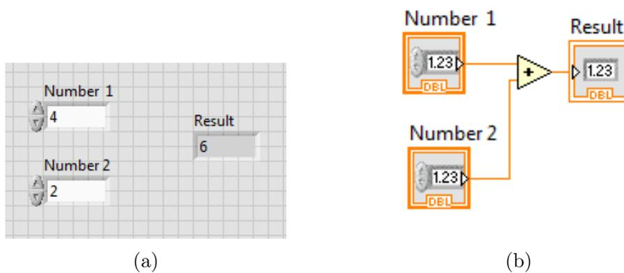
Figure 3.2: A simple VI in LabVIEW: (a) Front Panel, (b) Block Diagram.
