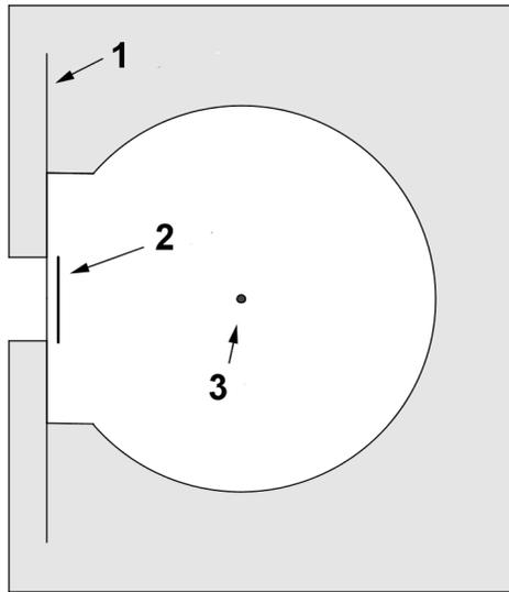
Figure 2.1: Schematic overview of the neutron detector. (1) neutron entrance window, (2) boron layer, (3) tungsten filament.
