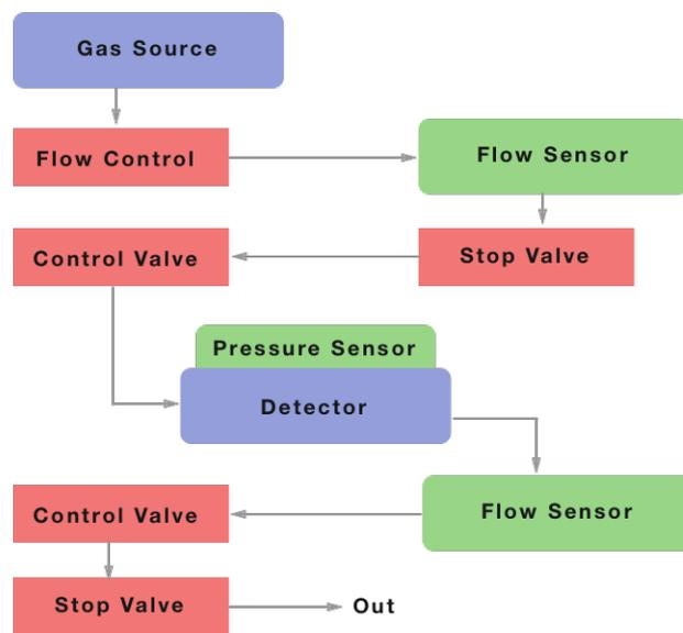
Figure 3.5: Overview of the gas system setup.
