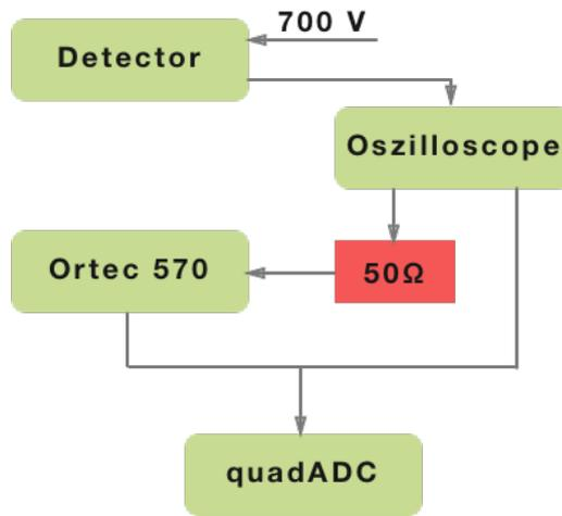
Figure 3.3: Structure of the electric setup.
